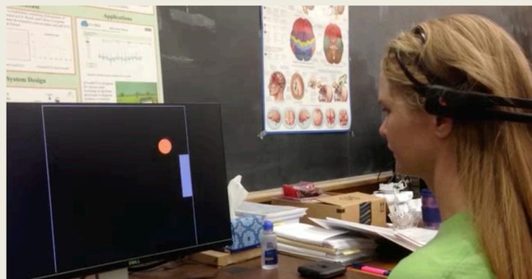
A picture captured during EEG-based Cursor Control experiments[2]
