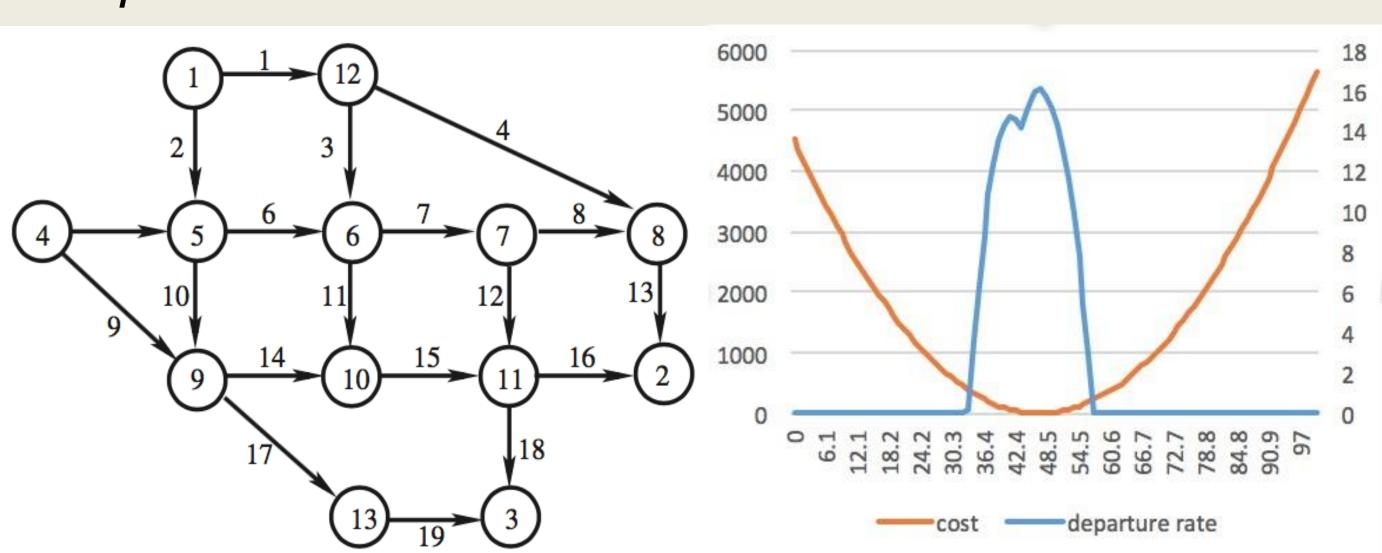
For the network as shown in the upper left graph, considering the characters of 19 different road, then the optimal choice of departure rate is presented in the graph in the upper right side.
