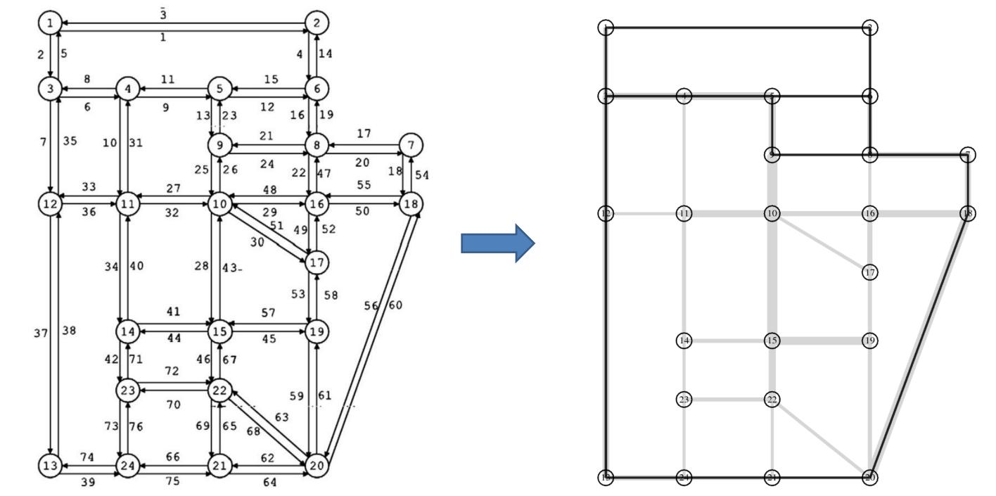
For the network as shown in the upper left graph, the assignment result can be shown on the graph. The running time can be reduced to one third compared with Frank-Wolfe algorithm in this example. GPU acceleration is significant.
