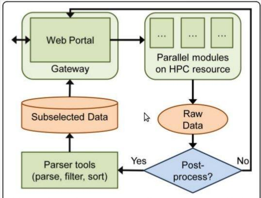
**Figure 2 The gateway approach**. The user interfaces with the science gateway portal and initiates a job that is run through parallel modules on an HPC resource. Based on the user's needs, either the raw results are delivered back to the user, or the output is parsed and prepared for easier use before it is made accessible through the gateway.
