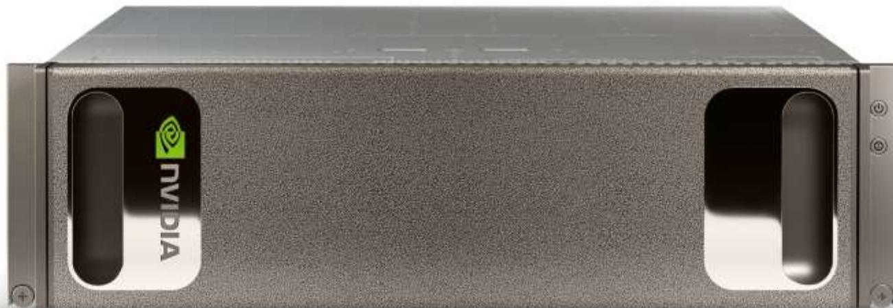
170 TFLOPS | 8x Tesla P100 16GB | NVLink Hybrid Cube Mesh
